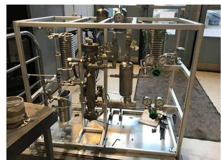
Laboratory set-up for MeOH synthesis
