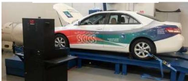
Chassis Dyno Drive Cycle Test
