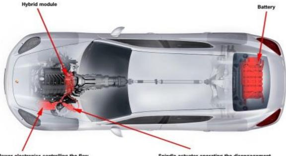
Power electronics controlling the flow of electric current between the battery and the electric motor Spindle actuator operating the disengagement clutch between the combustion engine and the electric motor
